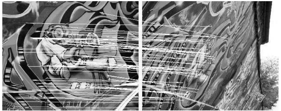
Figure 15: graffiti no.1 vs no.6, transition tilt t \sim 3.2 . Not shown: SIFT (0 match), Hessian-Affine (1 match).
