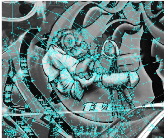
Figure 3: SIFT key points. The arrow starting point, length and the orientation signify respectively the key point position, scale, and dominant orientation. These features are covariant to any image similarity.
